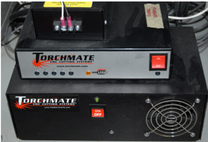
Signal Generator & Power Supply
