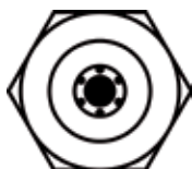
Nozzle DS channel's location
