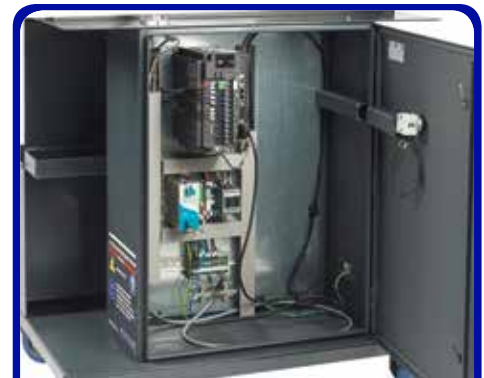
Sealed electrical box housing all NC Controls and cabling
