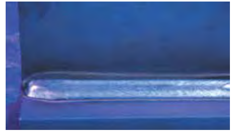
Horizontal fillet produced by Select 308L with CO 2 shielding gas. The bead is even and well-washed, with a finely rippled surface finish.
