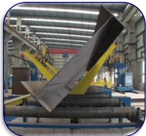
*Beam Flippers unit is assembled to the outfeed conveyor of Pull through welder which is used to flip the welded beam to other side for second side welding.*
